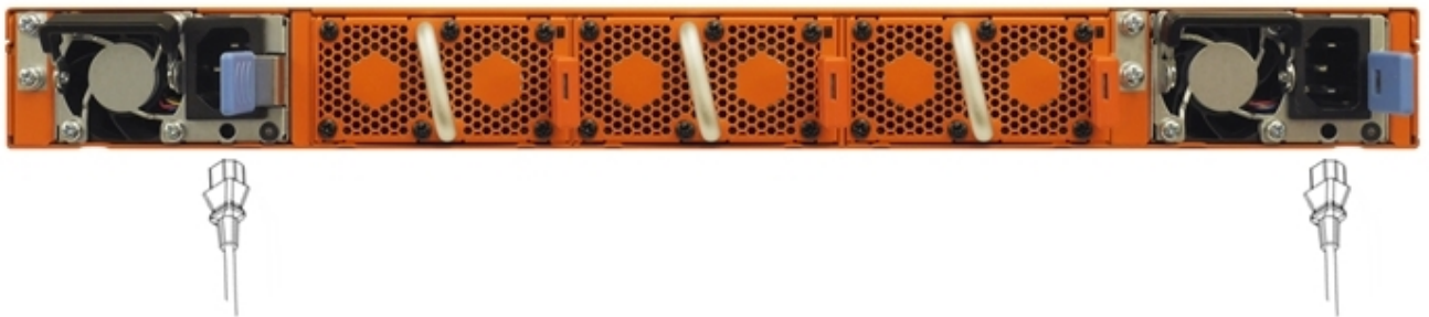
Figure 8 Connecting AC Power on a GigaVUE TA Series-TA100
